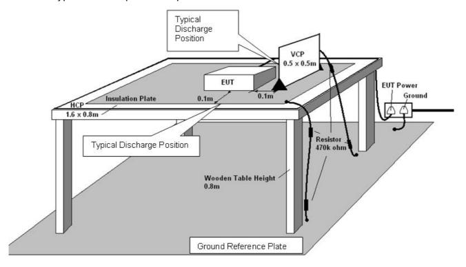
The typical floor-stand test setup is as follow:
