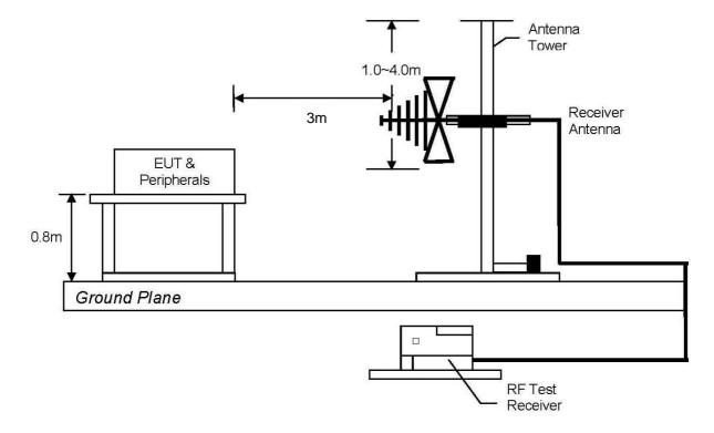
For tabletop equipment, the equipment under test was placed on the top of rotation table 0.8 meter above ground plane. For floor-standing equipment, the EUT and all cables were insulated, if required, from the ground plane by up to 12 mm of insulating material.
